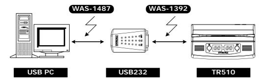
3. Communication between AC9400 access control RS-232 Device and USB Port
